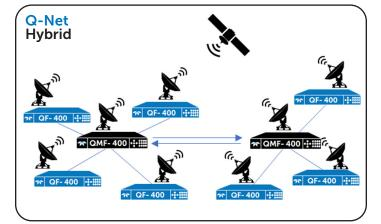
Q-Net Hybrid Network: In a Paradise Datacom point-to-multipoint network, the equipment is flexible enough to support hybrid topologies, allowing some nodes to have full access to other nodes, and some to communicate back to a hub. This can evolve as real-world networks evolve.
