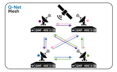
Full Mesh Network: A full hubless mesh network allows each remote site to communicate with all other remote sites, providing:
