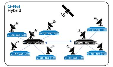
Q-Net Hybrid Network: In a Paradise Datacom point-to-multipoint network, the equipment is flexible enough to support hybrid topologies, allowing some nodes to have full access to other nodes, and some to communicate back to a hub. This can evolve as real-world networks evolve.
