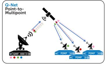
Q-Net Star Network: For a point-to-multipoint star network, the remote site transmits back to the hub, and the hub modem (QMultiFlex-400) is equipped with a separate demodulator for each site, up to a maximum of 16. However, a star system may be extended to support up to 128 sites with further QMultiFlex-400 demod only units connected at the hub. Each remote site communicates back to the hub or through the hub to other nodes. Remote sites can be populated with lower cost QFlex-400 P2MP modems.
