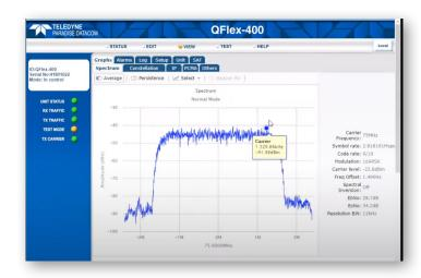
**Spectral view:** The Rx Spectrum Monitor is a powerful real-time spectrum analyser within the modem that is used to view the received signal spectrum. The monitor can not only display the wanted carrier but a Super Wide view allows checking for adjacent interfering carriers.
