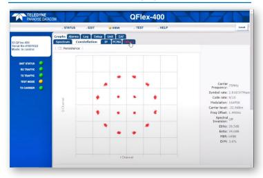
**Constellation view:** The Rx Constellation Monitor can be used to check for correct modem operation including checking for signal distortion and phase noise. The persistence mode is useful for showing any long-term effects due to phase noise and interference.
