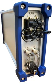
Rear of **Q-LiteE Rugged** modem showing weatherproof connectors (4 x Ethernet, Tx, Rx and DC input). A mounting bracket allows the modem to be secured in place. Several mounting options are available and can be customised to suit individual requirements.
