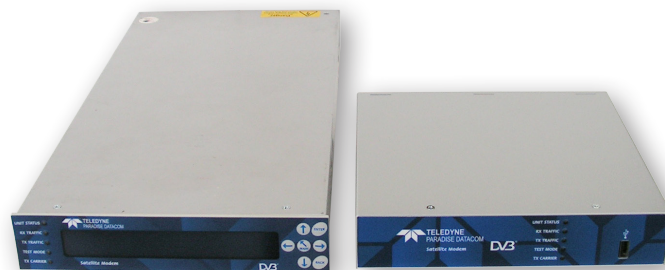
The AXIOM-C (right) is smaller than our Q-Lite Half-Width modem (left)
