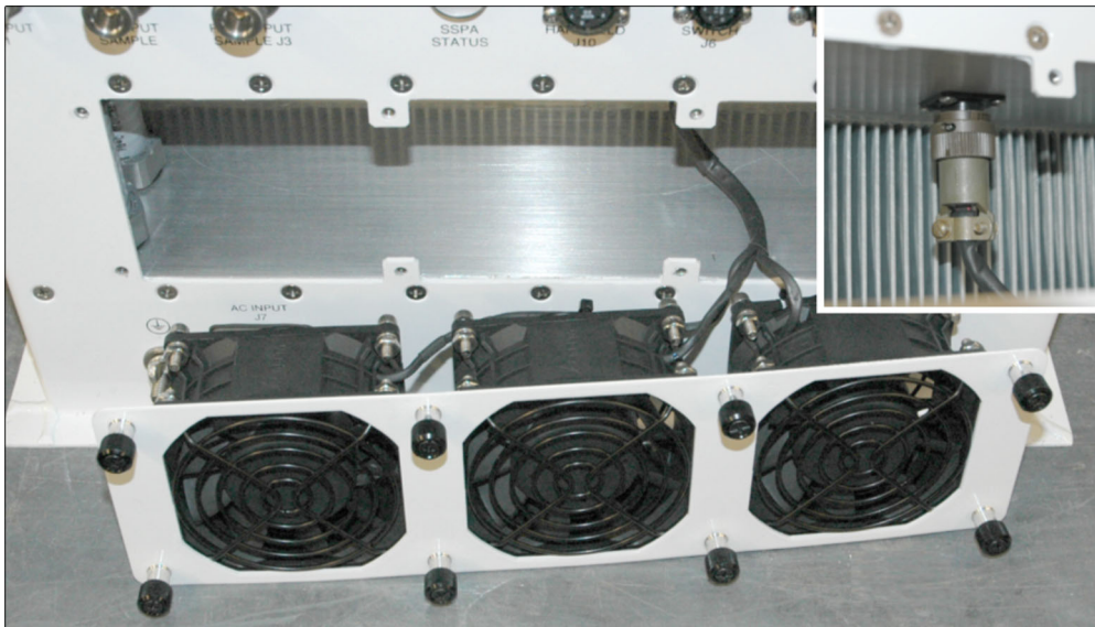
Figure 1: Intake Fan Assembly; inset, Fan Power Connector
