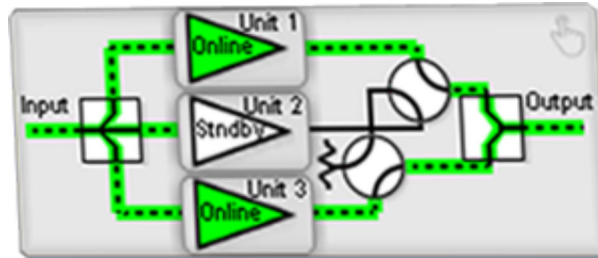
Figure 9: FPRC-1200 Mimic Display with HPA #2 in Standby Mode
