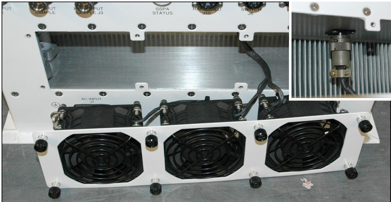
Figure 6-1: Intake Fan Assembly and Power Connector (inset)
