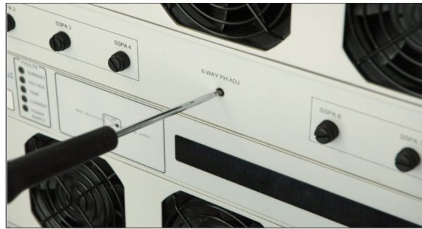
Figure 5: Adjust 8-Way Phase Trimmer
