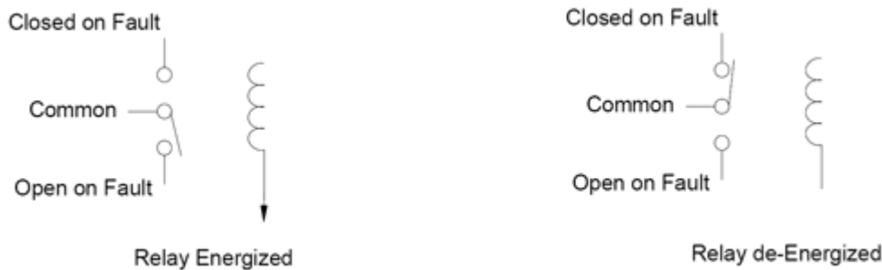
Figure 2: Parallel I/O Form-C Relay
