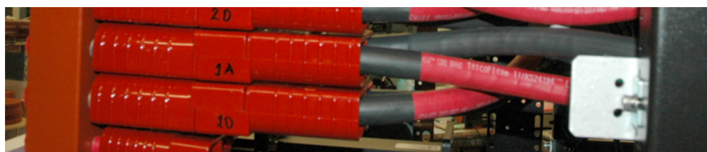
Figure 17: Connect Power Cables Between SSPA and Bus Rail
