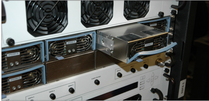
Figure 9: Install Power Supply Modules
