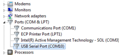
Figure 12: Firmware Upgrade, Check Device Manager for COM Port Designator
