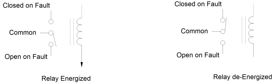
Figure 2: Parallel I/O Form C Relay
